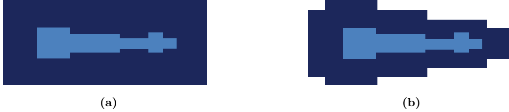
Figure 2 (a) The status-quo forging with weight x_0 for a component with weight 1, i.e., buy-to-fly ratio of x_0 -to-1, and (b) an improved forging with weight x for the same component, i.e., buy-to-fly ratio of x -to-1. In both panels, the light-colored area is the final component, and the dark-colored area is the scrap material the buyer will generate after machining, i.e., x_0 - 1 and x - 1 for the status-quo and improved designs, respectively.
